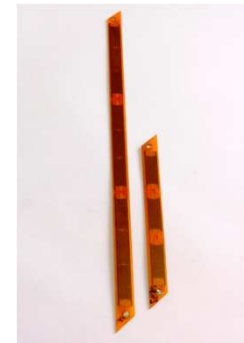
multilayer piezo-composites arrays into an active rotor blade
